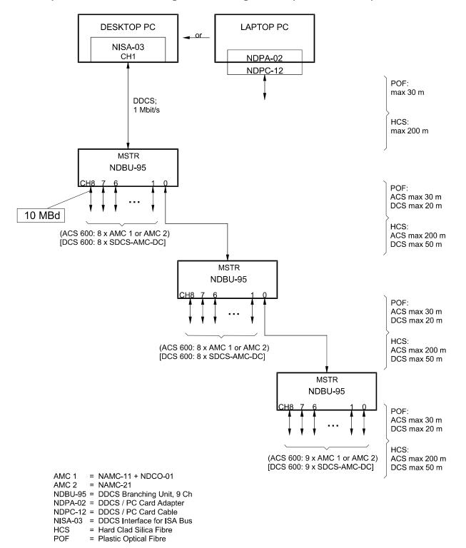
Example 2/3: Structure using a tree configuration (with NDBU-95)
