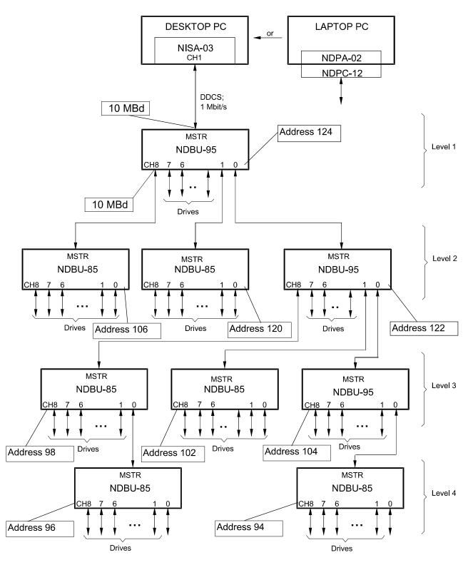
Example 2/5: Structure using a mixed configuration (with NDBU-85 and NDBU-95)
