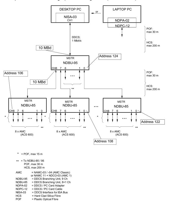
Example 2/2: Structure using a parallel configuration (with NDBU-85)
