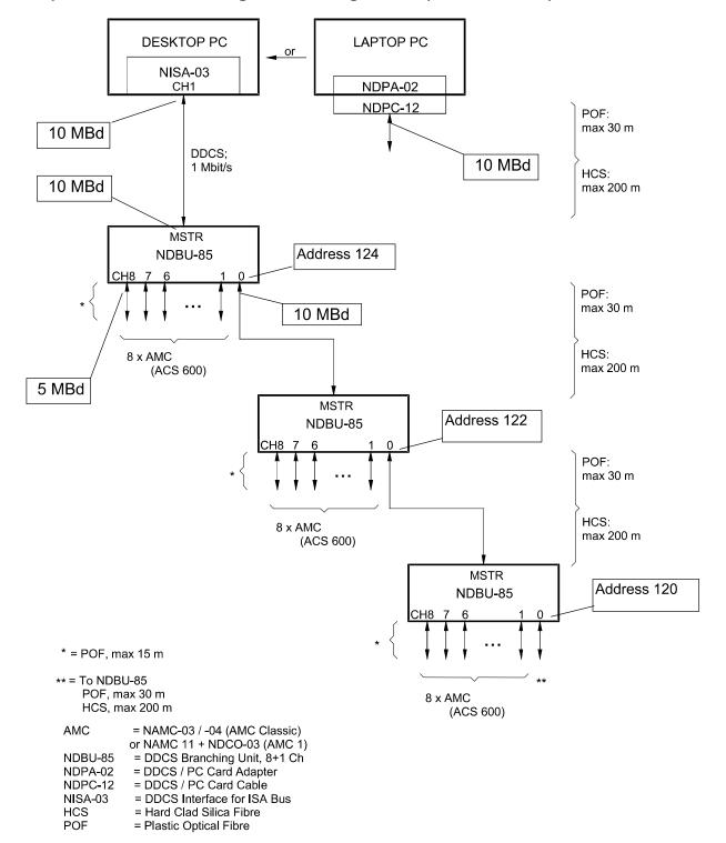
Example 2/1: Structure using a tree configuration (with NDBU-85)
