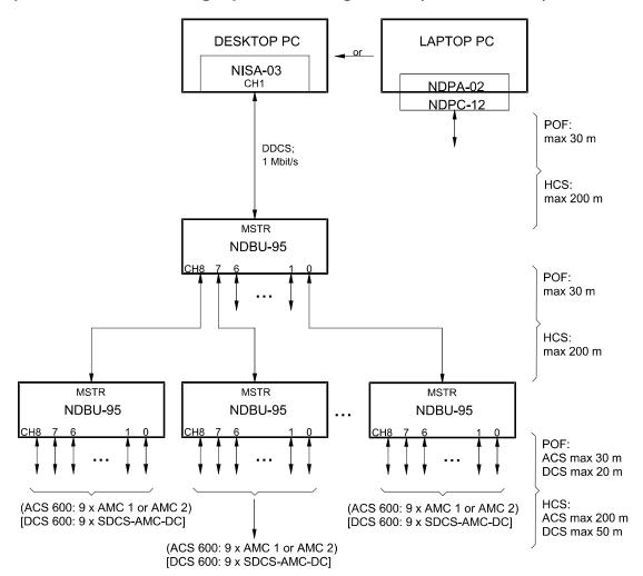
Example 2/4: Structure using a parallel configuration (with NDBU-95)
