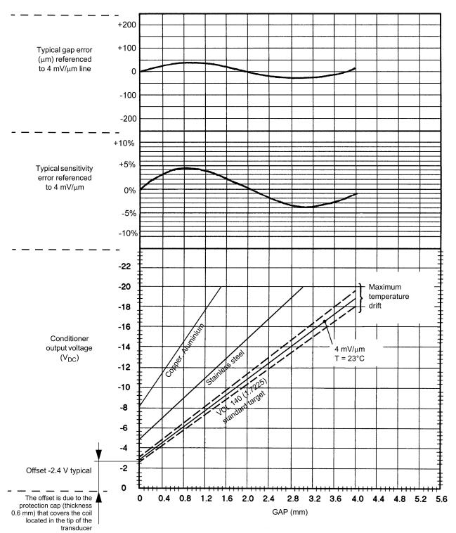
Proximity transducer: TQ 422 / TQ 432 Signal conditioner: IQS 452 Standard target material: VCL 140 (1.7225)
