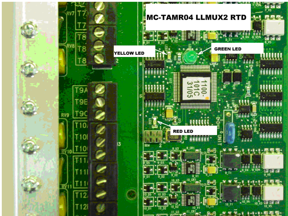
Figure 8.2 Location of Diagnostic LEDs on the LLMUX2 RTD FTA
