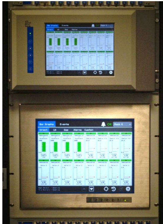
Figure 5: 10" Display Face Mount option (upper), 15" Display 19" EIA Rack Mount option (lower)
