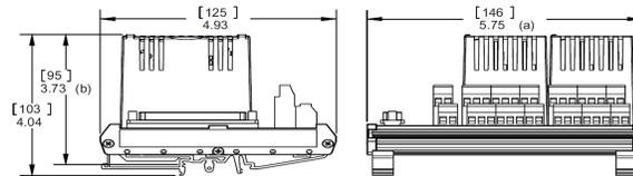
(a) Overall width – for determining DIN rail loading.
