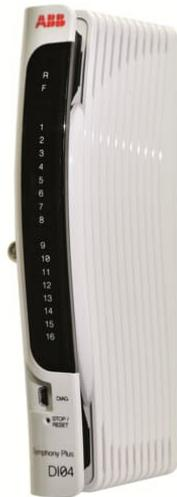
The DI04 digital input module processes up to 16 individual Digital Input signals. Each channel is individually CH-2-CH isolated and supports 48 VDC inputs. FC 221 (I/O Device Definition) sets DI module operating parameters and each input channel is configured using FC 224 (Digital Input CH) to set input channel parameters such as alarm state, debounce period, etc.
