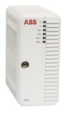
S800 I/O is a comprehensive, distributed and modular process I/O system that communicates with parent controllers and PLCs over industry-standard field buses. The TB840 ModuleBus Modem is a fiber optic interface to the Optical ModuleBus. TB840A is used in redundancy configurations where each module is connected to different optical ModuleBus lines, but connected to the same electrical ModuleBus.
