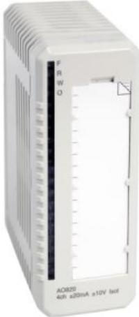
The AO820 Analog Output Module has 4 bipolar analog output channels. The choice of current or voltage output is configurable for each channel. There are separate sets of terminals for voltage and current outputs, and it is up to the user to wire outputs properly. The only differences between current or voltage channel configuration is in software settings.
