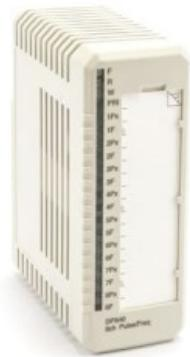
The DP840 module consists of 8 identical independent channels. Each channel can be used for pulse count or frequency (speed) measurement, maximum 20 kHz. The inputs can also be read as DI signals. Each channel has a configurable input filter. The module perform self-diagnostics cyclically. With advanced diagnostics, for single or redundant applications. Interface for NAMUR, 12 V and 24 V. The input can be read as digital input signals.
