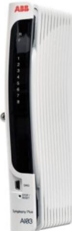
The AI03 Analog Input module processes up to 8 group isolated, RTD temperature input field signals. Each channel supports 2/3/4 Wire RTD wiring and is independently configurable for any of the supported RTD types. FC 221 (I/O Device Definition) sets AI module operating parameters and each input channel is configured using FC 222 (Analog Input Channel) to set individual input channel parameters such as engineering units, High/Low alarm limits, etc.
