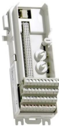
The TU818 is a 32 channel 50 V compact module termination unit (MTU) for the S800 I/O. The MTU is a passive unit used for connection of the field wiring to the I/O modules. It also contains a part of the ModuleBus.
